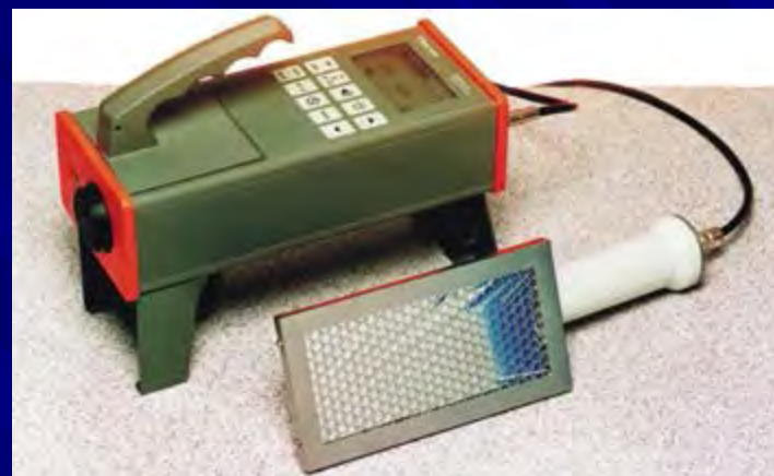
Thermo Electron Corp, Electra ratemeter with alpha probe
