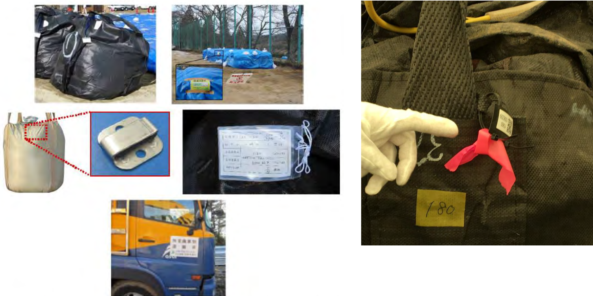
Figure 2-30: Flexible container and labelling system for packages and transport vehicles
