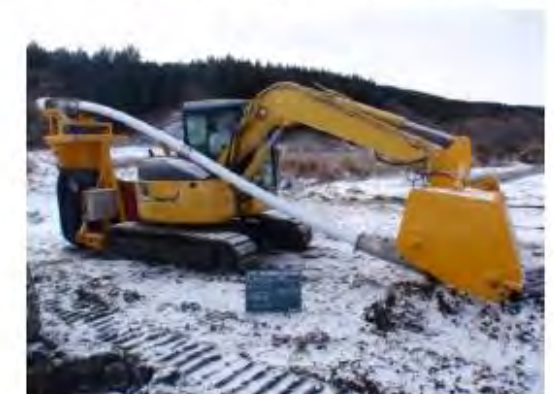
Solidified soil separation and recovery machine
