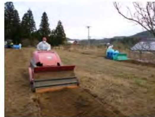
Thin layer topsoil stripper
