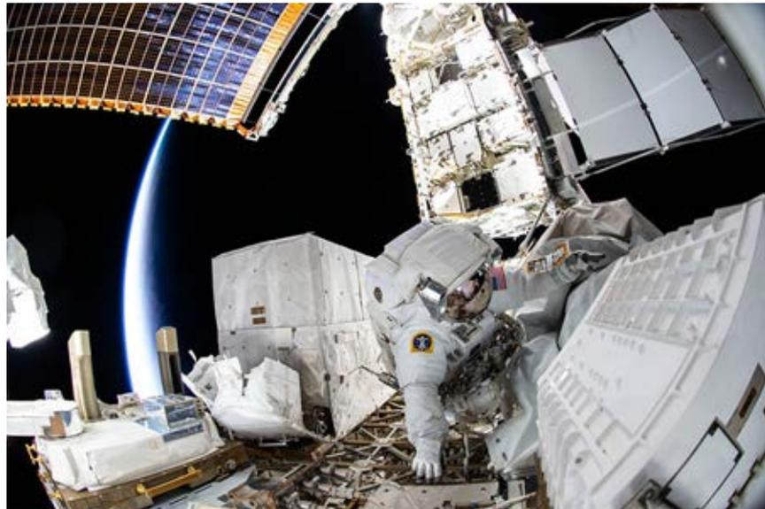
NASA spacewalker Kayla Barron is pictured during a 6 h and 32 min spacewalk to replace a failed antenna system on the International Space Station's Port-1 truss structure. <https://www.flickr.com/photos/nasa2explore/51732390695/>
