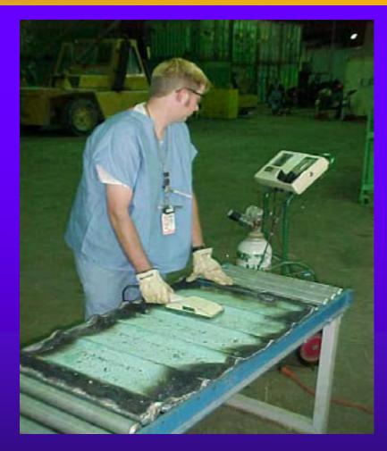
Surface contaminated metals can be decontaminated and/or surveyed for release (including recycling) if contamination is removed and verified by surveys.
