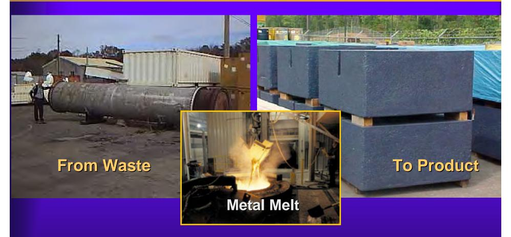
Contaminated metals can be recycled into useful radioactive products for use in radioactive material licensed activities and controlled programs.
